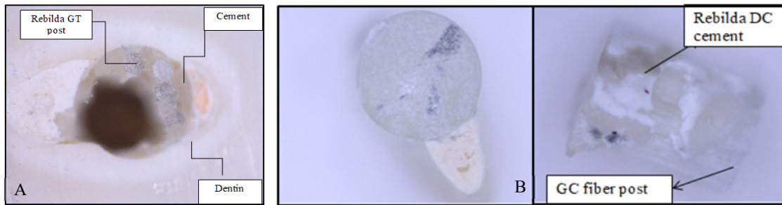
Figure 5: A - Mixed failure with resin cement covering the post surface and dentin, B - Mixed failure with resin cement covering the post surface and dentin (GC fiber post).
